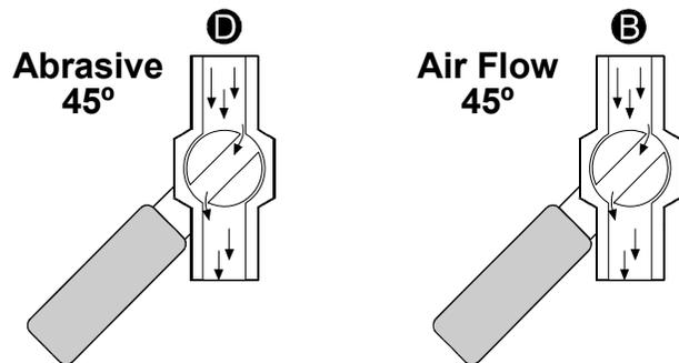
Set Air Flow Valve (B) approximately half way open or at 45° angle. Adjustments will need to be made as wear occurs to Blast Hose (K) and Blast Nozzle (T).
