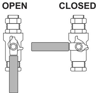
**3.1 Pressure Pot Settings:** The Pressure Pot has two adjustment ball valves that can regulate the abrasive/air flow mixture. The standard settings for the pressure pot should be made as follows:
