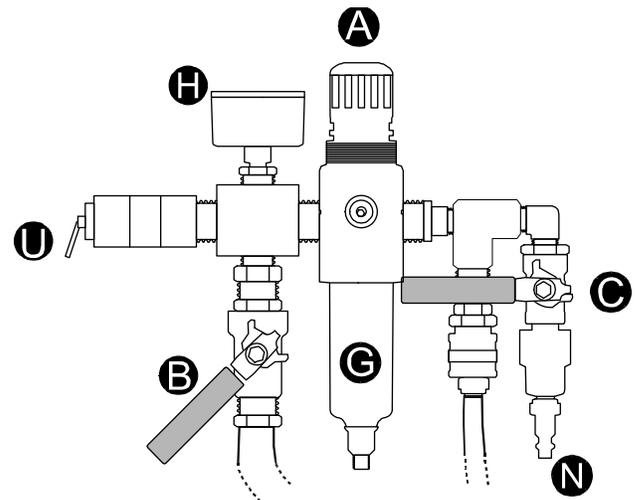
3.2.1 Before connecting the air hose from the compressor to the pot, make sure the Air Inlet Valve (C) is in the “OFF” position (horizontal) and the air compressor has been set up according to instructions found in the Rayzist setup guide.
