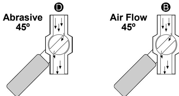
Set Air Flow Valve (B) approximately half way open or at 45° angle. Adjustments will need to be
