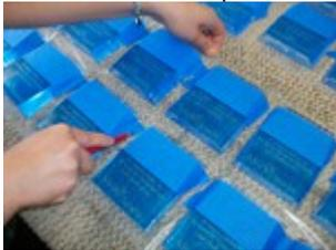
6. Apply four small strips of [blasting tape](#) to ensure no abrasive will work its way through the edge of the transfer tape.
