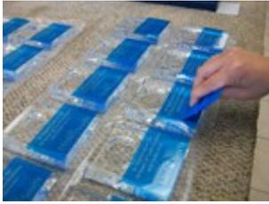
3. Remove the clear carrier on all of the photomasks and cover the front of each piece with blasting tape.
