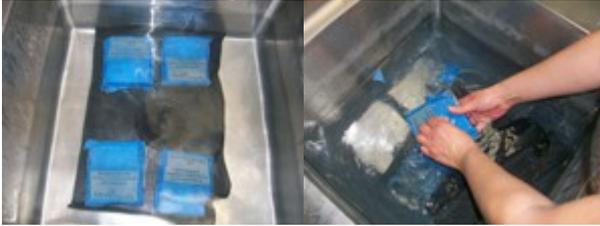
3. After you remove the photomask and tape, place the item in the third sink for the final rinse. If you allow the crystal to sit in warm water for a few minutes (or longer), the remaining bits of photomask and tape will come off easily.
