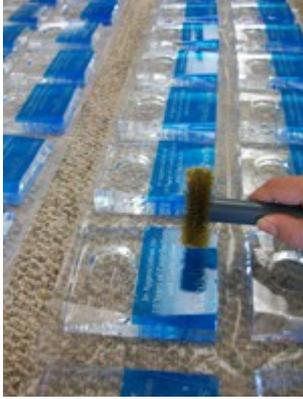
5. Cut the transfer tape between the crystal pieces with a razor or X-Acto knife. The transfer tape should fold up over each side of each piece and cover the entire blank.
